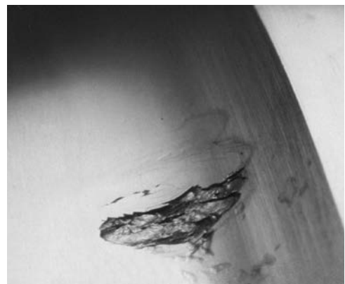
Fig. 5.2 Photo-illustration of fatigue damage on the raceway
